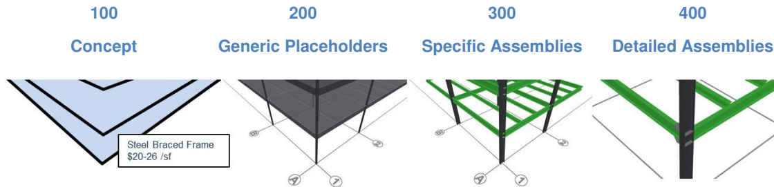
Figure 1 Steel Structure at Increasing LODs
